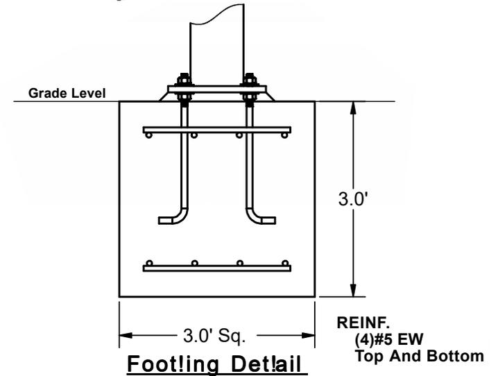
\*Footing design based on 1500 PSF soil bearing pressure.
