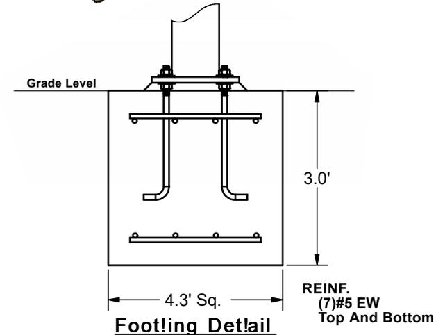
\*Footing design based on 1500 PSF soil bearing pressure.
