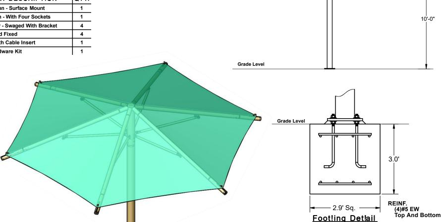
\*Footing design based on 1500 PSF soil
