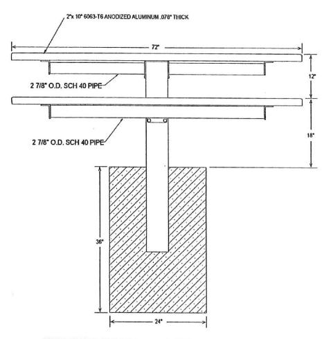
THE SIZE OF THE CONCRETE BASE IS ONLY A SUGGESTION YOUR LOCAL SOIL CONDITIONS SHOULD DETERMINE WHAT IS NECESSARY TO ENSURE A STABLE MOUNTING
