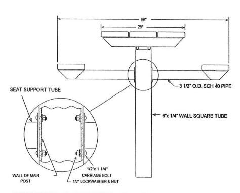
OUTSIDE ONLY SMOOTH CARR. BOLT HEADS ARE EXPOSED THE LOCKWASHERS & NUTS ARE ON THE INSIDE OF THE MAIN POST SO WHEN THE TABLE IS FULLY ASSEMBLED THEY ARE NOT ACCESIBLE
