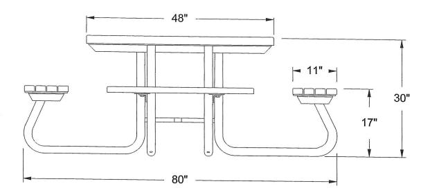
The frame is made from heavy 1 5/8" OD pipe. A heavy X brace stabilizes the whole frame. It is coated with a long lasting powdercoat in black. The top and seats are 2" x 3" nominal recycled plastic that is UV protected. The recycled plastic is steel reinforced to prevent sagging.
