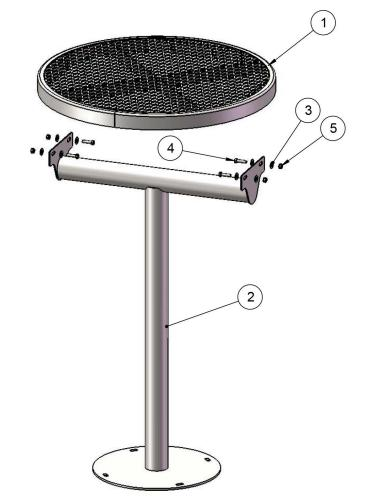
Required surface mount hardware: 3/8" x 3" concrete expansion anchor bolts (not included)
