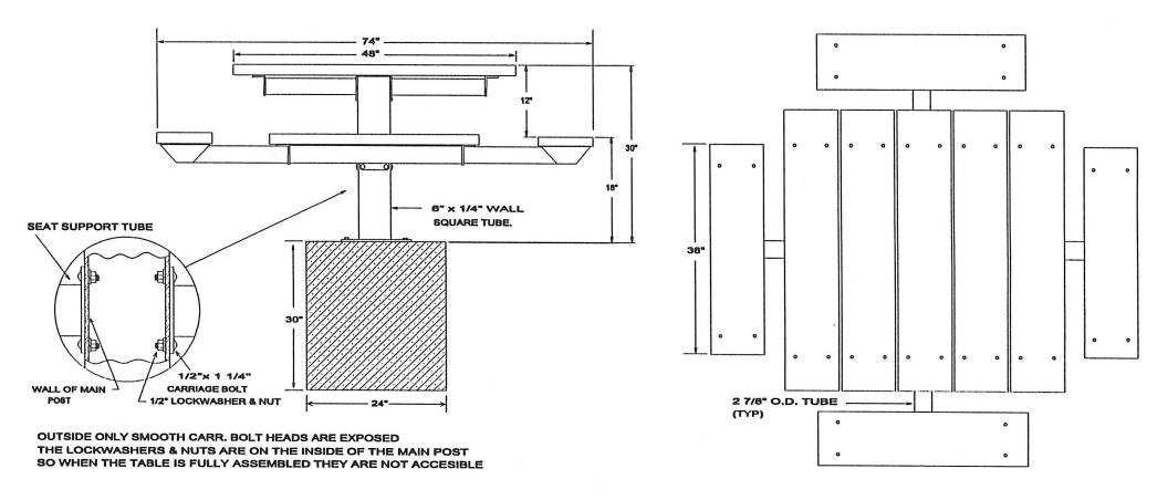
THE SIZE OF THE CONCRETE BASE IS ONLY A SUGGESTION YOUR LOCAL SOIL CONDITIONS SHOULD DETERMINE WHAT IS NECESSARY TO ENSURE A STABLE MOUNTING
