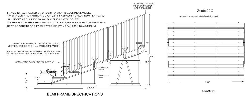
THESE FRAMES ARE DESIGNED AND TESTED TO BE IN ACCORDANCE WITH FEDERAL SPEC # RR-B-425-C
